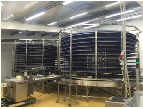
Our system is designed with 2 luffing conveyors to enable the products to be diverted from the line to the spiral accumulation system, to be held there until the main line is up and running again and then to be moved back onto the line once the problem at the packing end is fixed and the line is moving again.
